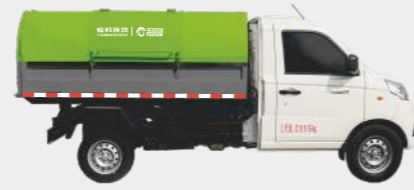
Sealed self dumping garbage truck
