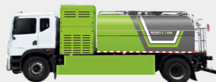
Hydrogen fuel cell sprinkler
