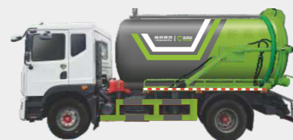
Sewage suction truck
